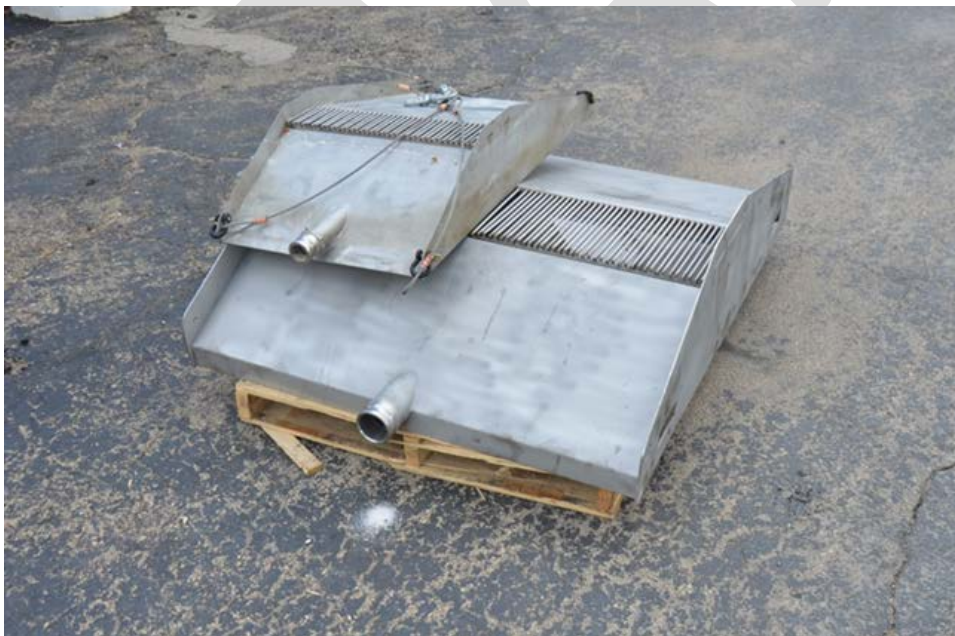
Figure 5. Two and four foot-wide collectors used in the Mackinaw River Study
