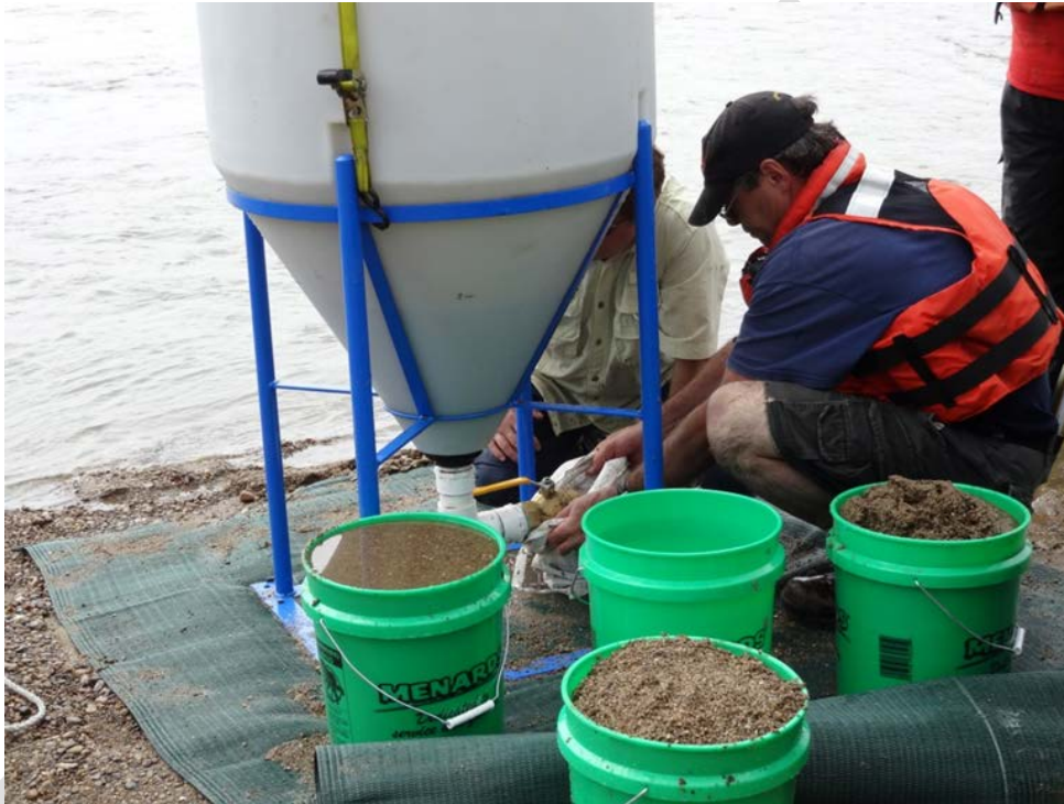
Figure 8. Harvested sediment being retrieved in a filter cloth bag from settling tank
