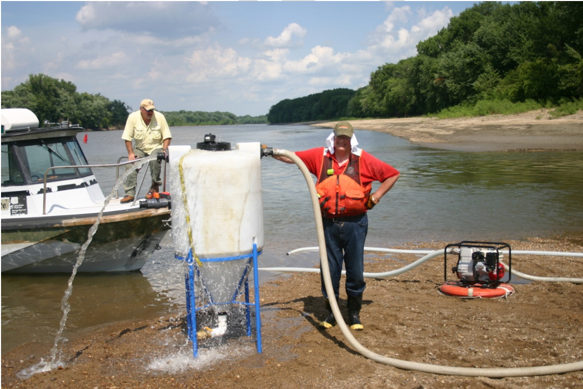
Figure 7. Pump and settling tank assembly
