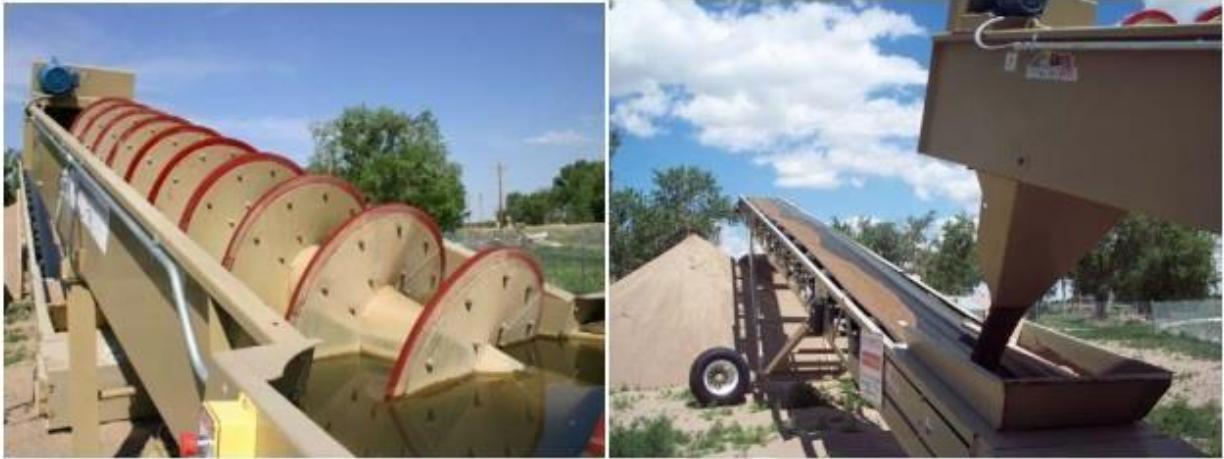
Figure 7: Image of supporting infrastructure to transport sediment and slurry from hopper to staging area (Streamside 2020).
