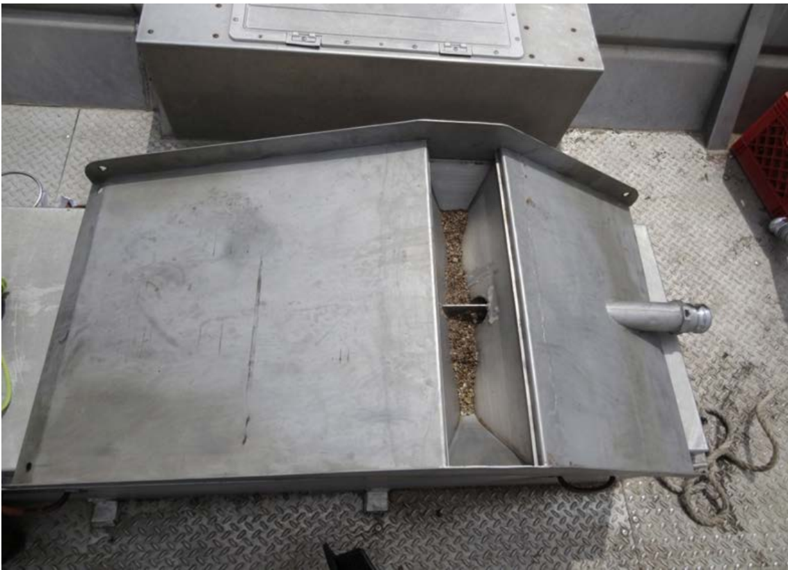
Figure 6. Four foot collector with grate off to show hopper, hopper suction port, and pipeline fitting
