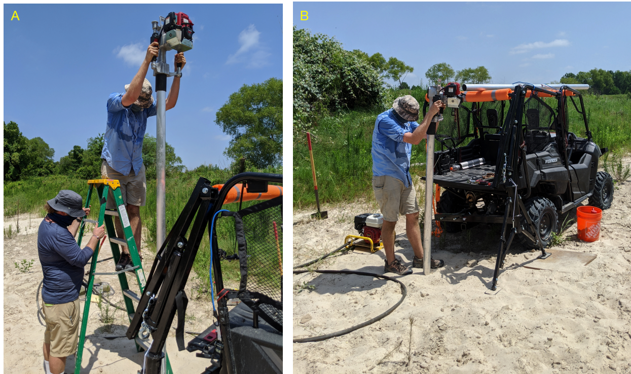
Figure 2. A) Pile driver being used to drive in core barrel at ST003 site B) Pile driving being driven in, with vibra-corer on ground next to student and UTV in background.
